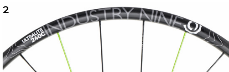
2015-19 UltraLite 240 Carbon | Rim + Graphic Change 23.5mm IW | 29" ERD 599 24H 29" DS 299mm | Non-DS 295mm
