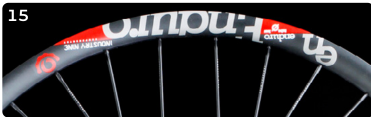
2013-14 Enduro Alloy 26mm IW | 26" ERD 532 | 27.5" ERD 560 | 29" ERD 597 32H 26" DS 266mm | Non-DS 268mm 32H 27.5" DS 278mm | Non-DS 280mm 32H 29" DS 297mm | Non-DS 299mm
