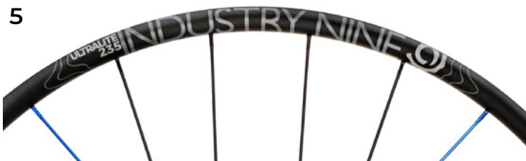
2017-19 UltraLite 235 Alloy | Rim + Graphic Change 23.5mm IW | 27.5" ERD 563 | 29" ERD 602 24H 27.5" DS 281mm | Non-DS 277mm 24H 29" DS 300mm | Non-DS 296mm
