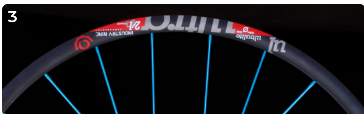
2013-14 UltraLite Alloy 21.3mm IW | 26" ERD 536 | 27.5" ERD 561 | 29" ERD 599 24H + 32H 26" 269mm | Non-DS 265mm 24H + 32H 27.5" 281mm | Non-DS 277mm 24H 29" DS 300mm | Non-DS 296mm 32H 29" DS 298mm | Non-DS 300mm
