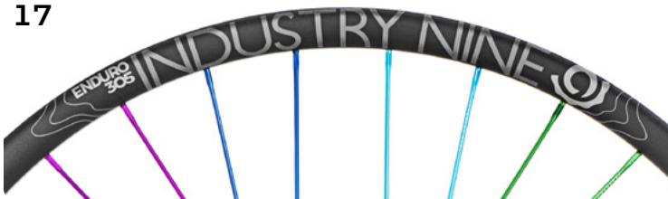
2017-19 Enduro 305 Alloy | Graphic Change 30.5mm IW | 26" ERD 532 | 27.5" ERD 560 | 29" ERD 597 32H 26" DS 266mm | Non-DS 268mm 32H 27.5" DS 278mm | Non-DS 280mm 32H 29" DS 297mm | Non-DS 299mm
