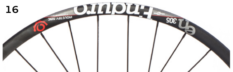
2015-16 Enduro 305 Alloy | Rim + Graphic Change 30.5mm IW | 26" ERD 532 | 27.5" ERD 560 | 29" ERD 597 32H 26" DS 266mm | Non-DS 268mm 32H 27.5" DS 278mm | Non-DS 280mm 32H 29" DS 297mm | Non-DS 299mm
